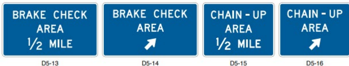
Figure 2I-6. Brake Check Area and Chain-Up Area Signs
