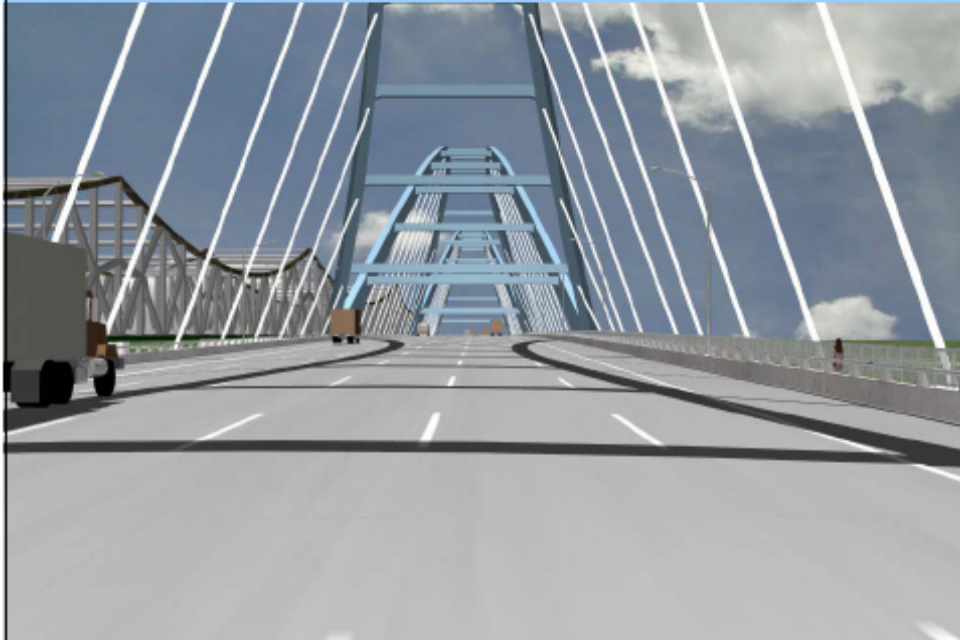
ALTERNATIVE 2: THREE SPAN THRU ARCH
