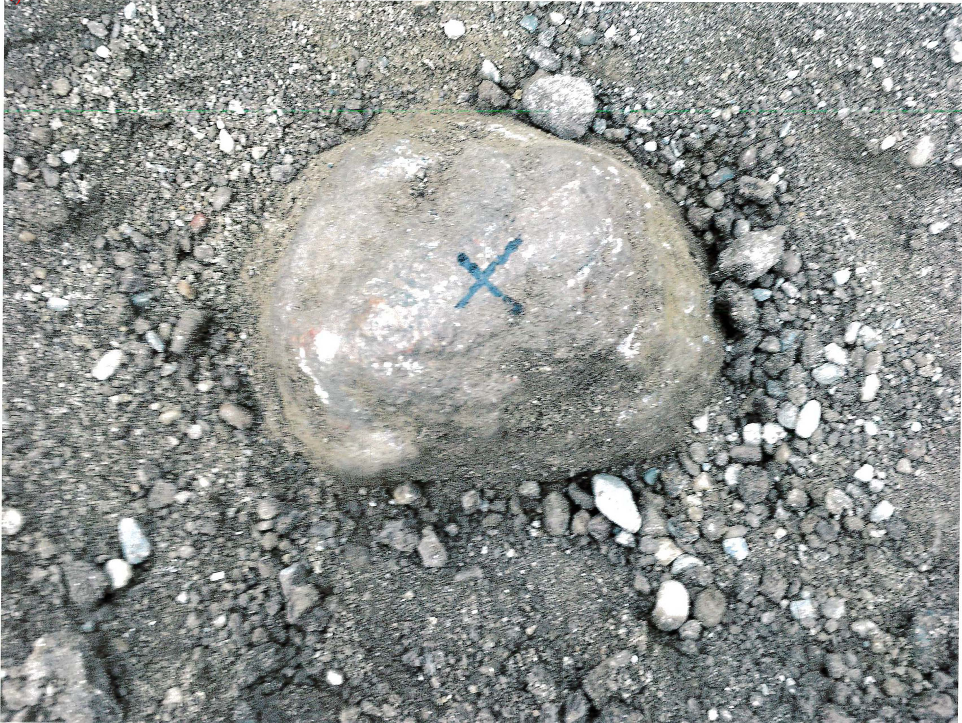
10"x9" Boulder 12" below gravel @ SE 24, NE 25, T11N, R5E Set rebar angled over peak N 1504167.50 E 258238.39
