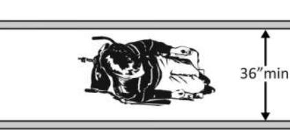
A diagram showing a person in a wheelchair using a narrow route between two parallel lines. A vertical double-headed arrow indicates a height of 36" min.                                                                                                                                                                          | N/A<br>Photo #: | <ul style="list-style-type: none"> <li>Widen route</li> <li>•</li> <li>•</li> </ul>                                                      |
