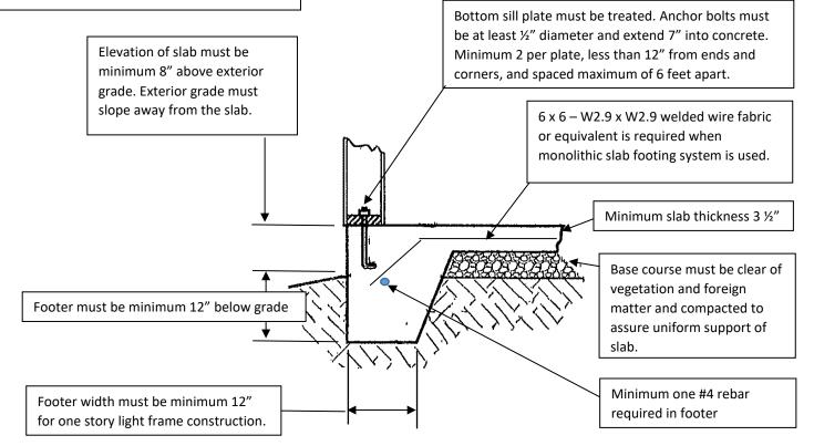
Note: If footer is poured separately from slab, then ½" horizontal rebar required in footer and in slab above footer. Vertical #3 rebar 48" on center required to tie slab into footer.
