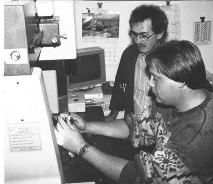
Bill Schribner, owner of Detail Tool & Die, and Greg Walls are shown operating a coordinate measuring machine, which is used for quality inspection of manufactured parts. The 29-year-old business has been in its current location 20 years. They design and manufacture plastic injection molds for companies in the U.S. and Mexico.
