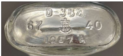
Some bottles have their manufacture and content information incorporated as part of their design. This glass bottle base shows a distiller number ("D-388") and bottle maker (the H-and-anchor motif represents the Anchor-Hocking Glass Company) as well as other identifying information. In this case, the markings tell us the bottle once held whiskey and most likely dates to c. 1940. Photo courtesy of DHPA.
