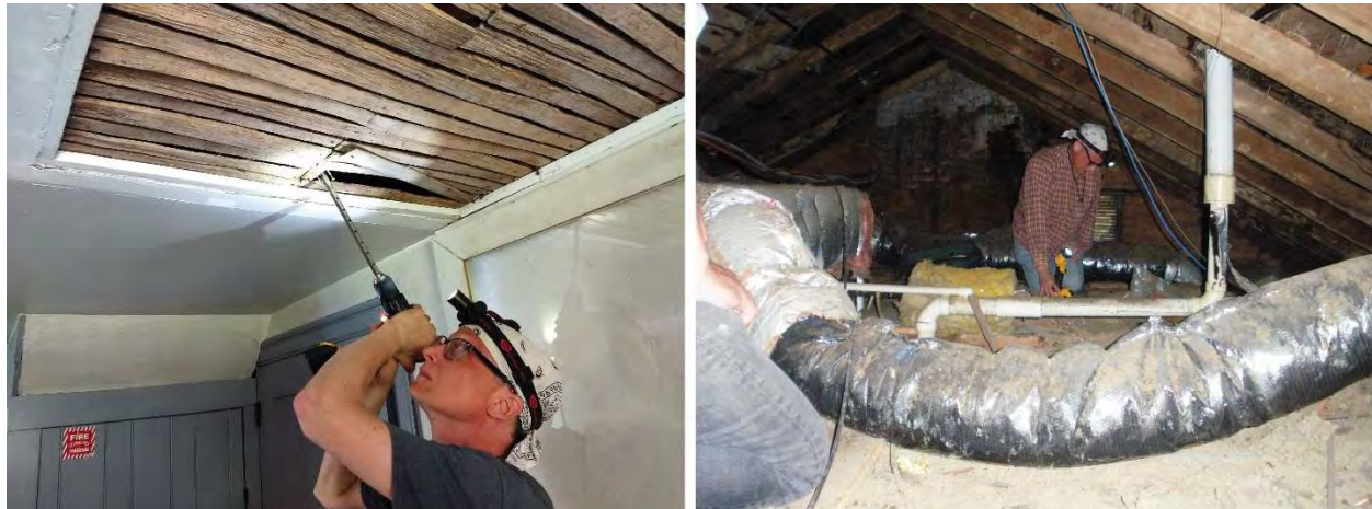
Figure 10. Sampling locations were limited in the Huddleston house. An exhibit interpreting traditional lath and plaster construction methods in the ceiling was partially dismantled to obtain sample HHH01 (left). The wood frame and a clear plastic panel were removed to gain access to a joist that was accessible through individual pieces of lath. Sampling rafters in the attic to obtain samples HHH04A through HHH05B (right) (Photo credit: Christopher Baas).
