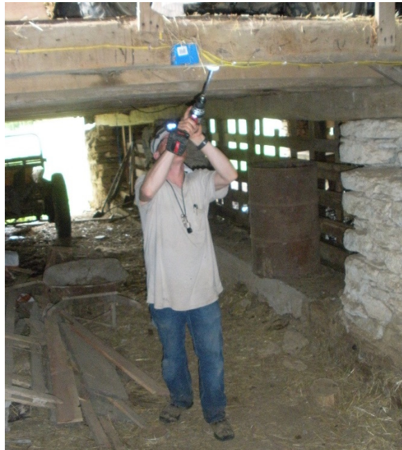
Figure 12. Core samples were obtained using a drill and dry wood boring bit. Photo courtesy of Christopher Baas.
