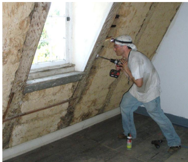
Figure 10. Core samples were obtained using a drill and dry wood boring bit (photo courtesy of Christopher Baas).
