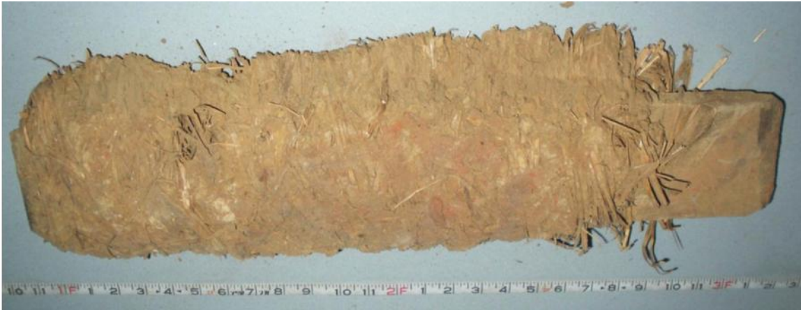
Figure 7. Dutch biscuit—a short wood plank wrapped in mud and straw (photo courtesy of Christopher Baas).
