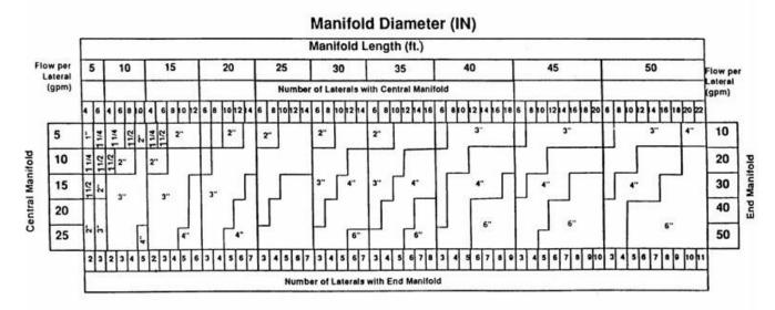
Computed for Plastic Pipe Only. The Hazen-Williams equation was used to compute headlosses through each segment (Hazen-Williams C h-150). The maximum manifold length for a given lateral discharge rate and spacing was defined as that length at which the difference between the heads at the distal and supply ends of the manifold exceeded 10 percent of the head at the distal end.
