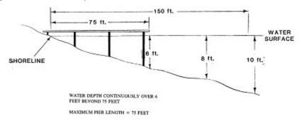
Where the maximum water depth is continuously more than six (6) feet beyond seventy-five (75) feet from the shoreline, the maximum pier length is seventy-five (75) feet.
