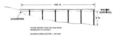
Where the water depth is six (6) feet or less from the shoreline to one hundred fifty (150) feet from the shoreline, the maximum pier length is one hundred fifty (150) feet.
