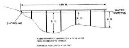
Where the maximum water depth is not continuously over six (6) feet from the shoreline, the maximum pier length is one hundred fifty (150) feet.
