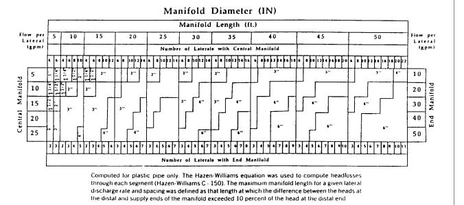
(v) The minimum inside diameter of the distribution pipes from the delivery manifold shall be one (1) inch; the maximum inside diameter of the distribution pipes shall be three (3) inches.
