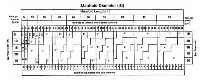
Computed for Plastic Pipe Only. The Hazen-Williams equation was used to compute headlosses through each segment (Hazen-Williams C h-150). The maximum manifold length for a given lateral discharge rate and spacing was defined as that length at which the difference between the heads at the distal and supply ends of the manifold exceeded 10 percent of the head at the distal end.
