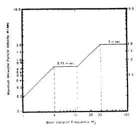
If the chart limits are used, a seismographic record including both particle-velocity and vibration-frequency levels shall be obtained for each blast. The method for the analysis of the predominant frequency contained in the blasting records shall be approved by the director before application of this alternative blasting criterion.
