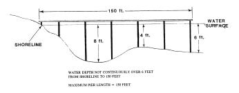
Where the maximum water depth is not continuously over six (6) feet from the shoreline, the maximum pier length is one hundred fifty (150) feet.
