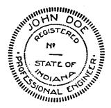
Plans containing an engineer seal of specified size may be reduced as long as the seal remains legible.
