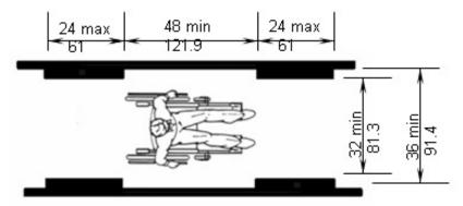
Figure 9 Clear Width of an Accessible Route
