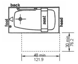
Figure 8 Alternative Specification – Clear Floor Space at Bathtub
