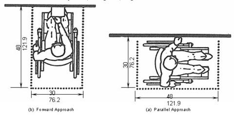
Figure 6 Minimum Clear Floor Space for Wheelchairs
