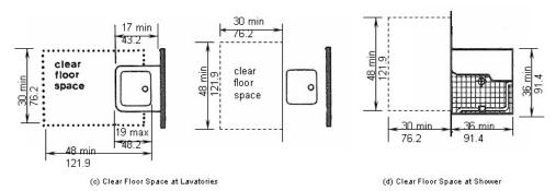
Figure 7 Clear Floor Space for Adaptable Bathrooms
