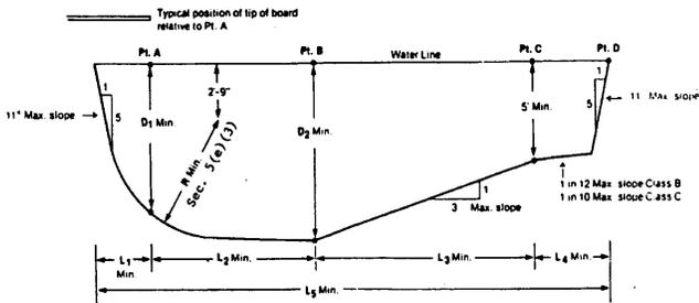
NOTE: L4 is a minimum dimension to allow sufficient length opposite the board. This must be lengthened to form the shallow portion of the pool
