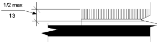
Fig. 302.2 Carpet on Floor Surfaces
