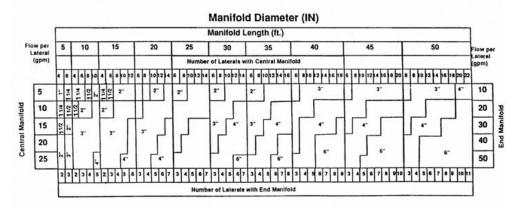
Computed for Plastic Pipe Only. The Hazen-Williams equation was used to compute headlosses through each segment (Hazen-Williams C<sub>h</sub>-150). The maximum manifold length for a given lateral discharge rate and spacing was defined as that length at which the difference between the heads at the distal and supply ends of the manifold exceeded 10 percent of the head at the distal end.
