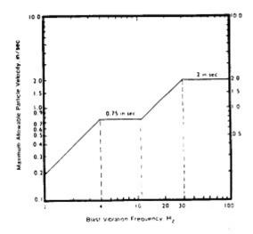
If the chart limits are used, a seismographic record including both particle-velocity and vibration-frequency levels shall be obtained for each blast. The method for the analysis of the predominant frequency contained in the blasting records shall be approved by the director before application of this alternative blasting criterion.
