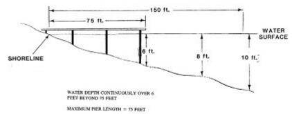
Where the maximum water depth is continuously more than six (6) feet beyond seventy-five (75) feet from the shoreline, the maximum pier length is seventy-five (75) feet.
