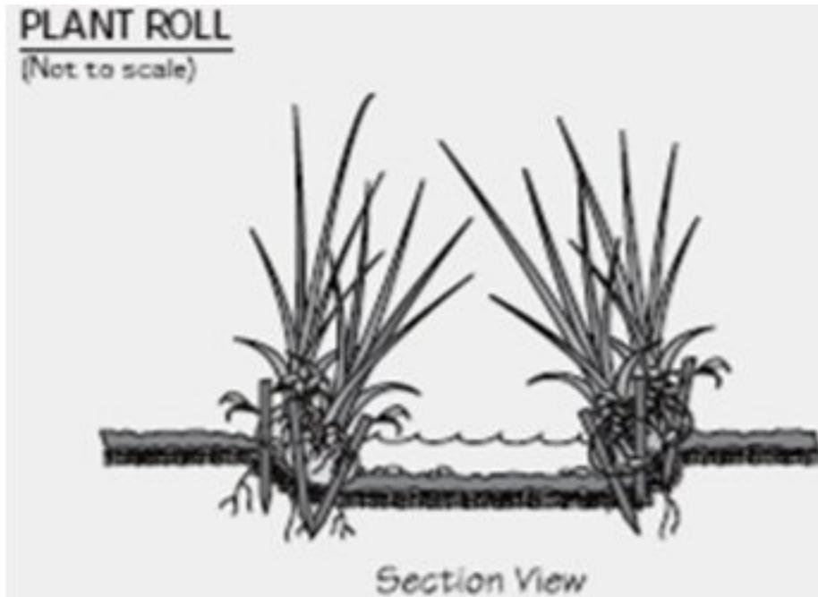
Ideal places for plant rolls are in areas where rapid repair of minor damage is needed. Many native species can grow in a plant roll, including many species of sedges, rushes, and grasses. Rolls are ideal where these types of plants normally grow. Unlike seeding, plant rolls can withstand areas of fluctuating water. Because rolls collect sediment and improve the microclimate, native species can easily become established and survive around a roll. Rolls offer immediate toe protection.
