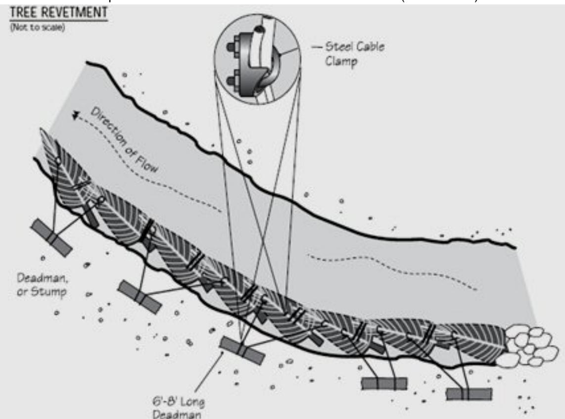
Log, root wad, and boulder revetments are a combination of bioengineered materials using the ideas from log revetments and boulder revetments. This technique is often used when added erosion protection is needed (USDA 2002).
