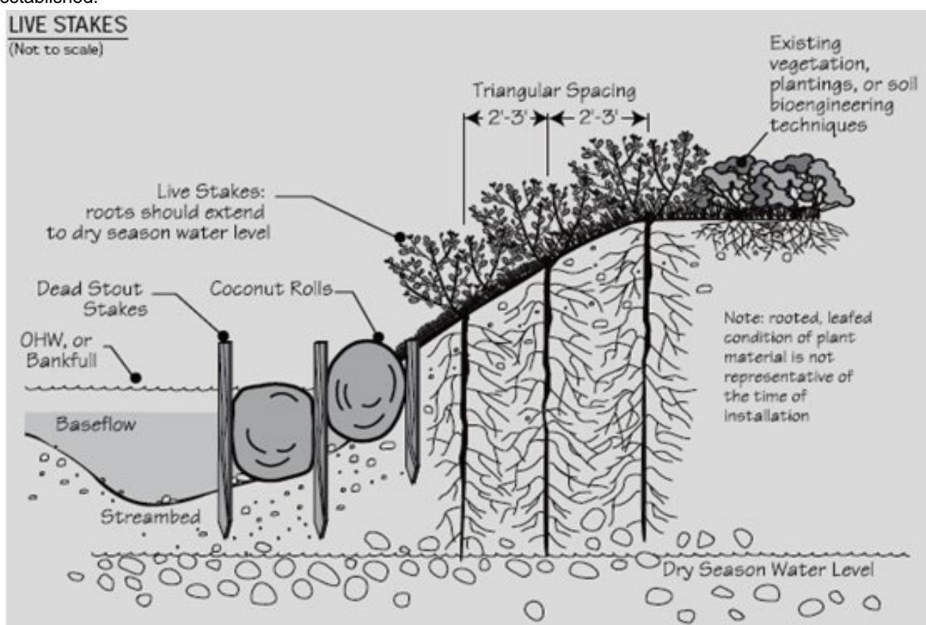
Live stakes can be installed in conjunction with other bioengineering materials, such as geotextile fabric, coconut fiber logs, and live fascines. If a streambank is exceptionally prone to erosion, laying geotextile with the live stakes helps control erosion while the live stakes take root. Live posts are quite similar to live stakes, only live posts are much larger (USDA 2002).
