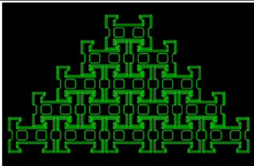
Cellular concrete blocks offer hard armor with voids to allow vegetation to become established, thereby providing wildlife habitat and an aesthetically pleasing condition. The blocks can be laid by hand which reduces additional site disturbance and allows their application in areas inaccessible to heavy machinery. The system provides a safe surface for pedestrians and wildlife.
