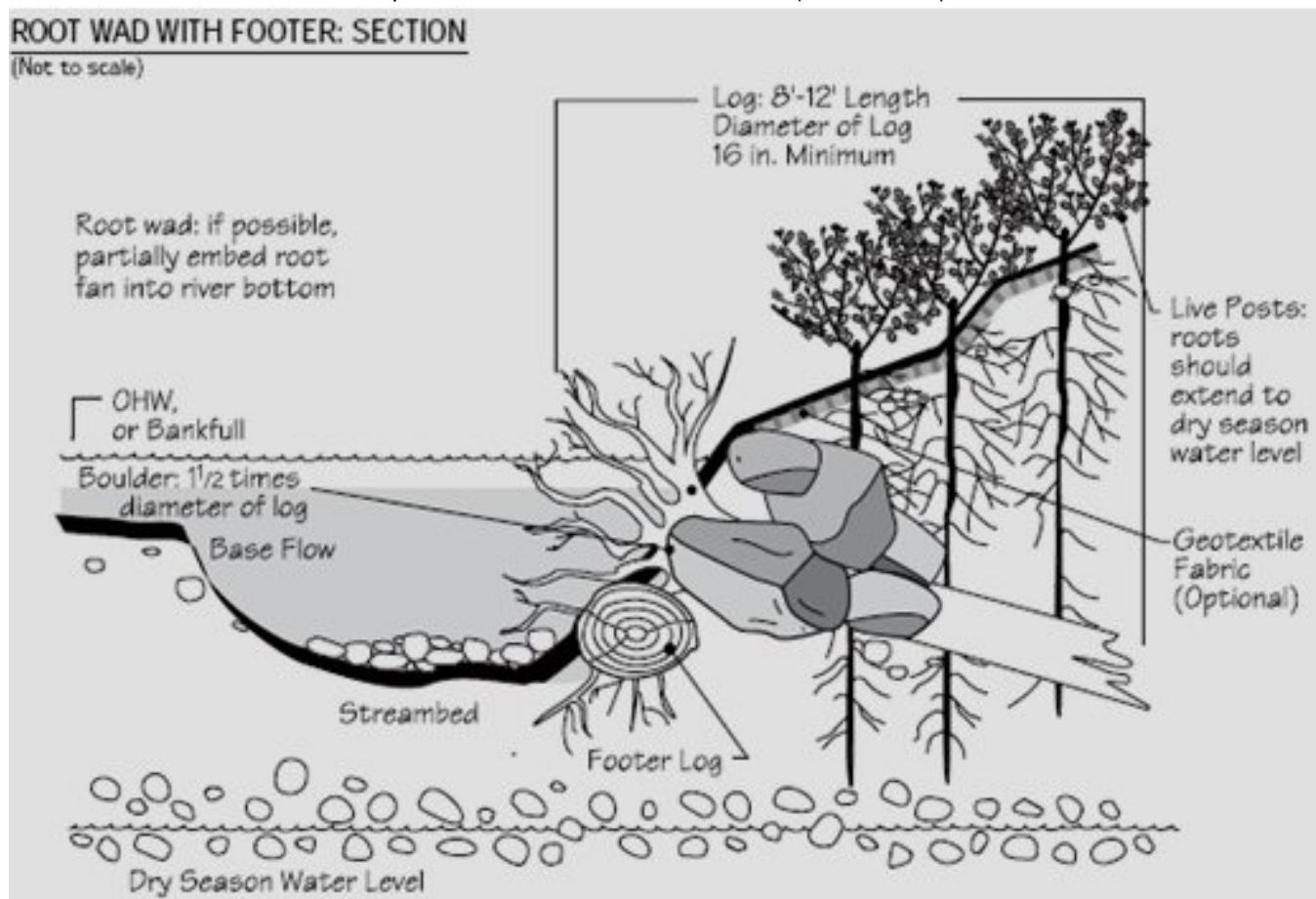
Most root wads are quite large and require heavy machinery for installation, which can cause increased stream sedimentation (Alaska Department of Fish and Game 2005). Use is also site-limited. If undercutting is likely, root wads should not be used. Also, they cannot be used in braided streams or with sandy or silty soil. Regular monitoring is required since they can decay or become damaged (MDE 2000).
