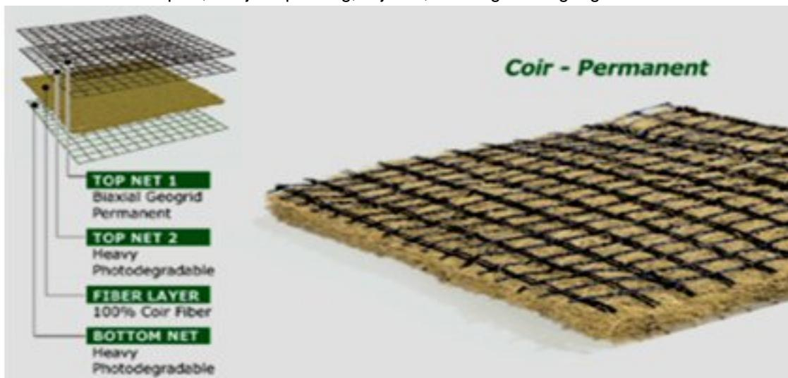
Turf reinforcement mats (TRMs) are manufactured coverings used to provide bank stabilization and prevent erosion. Generally, they are blankets of organic mulch distributed between fiber netting. The netting can be photodegradable polypropylene, a biodegradable natural fiber netting, or a more permanent material such as
