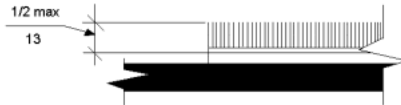
Fig. 302.2 Carpet on Floor Surfaces
