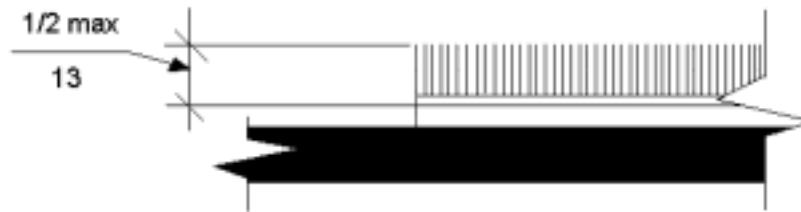
Fig. 302.2 Carpet on Floor Surfaces
