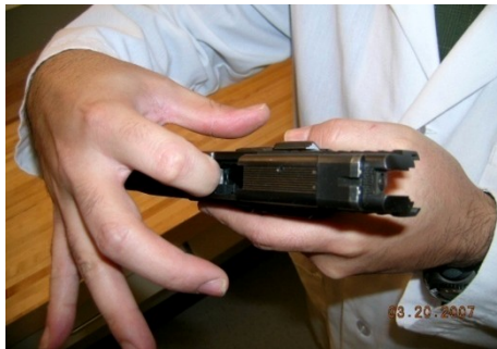
Step 5: Physically inspect the chamber
