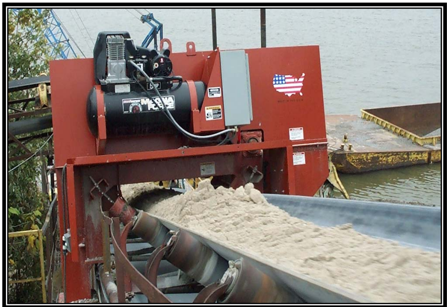
Figure 9-2. Belt Sampling with Mechanical Device
