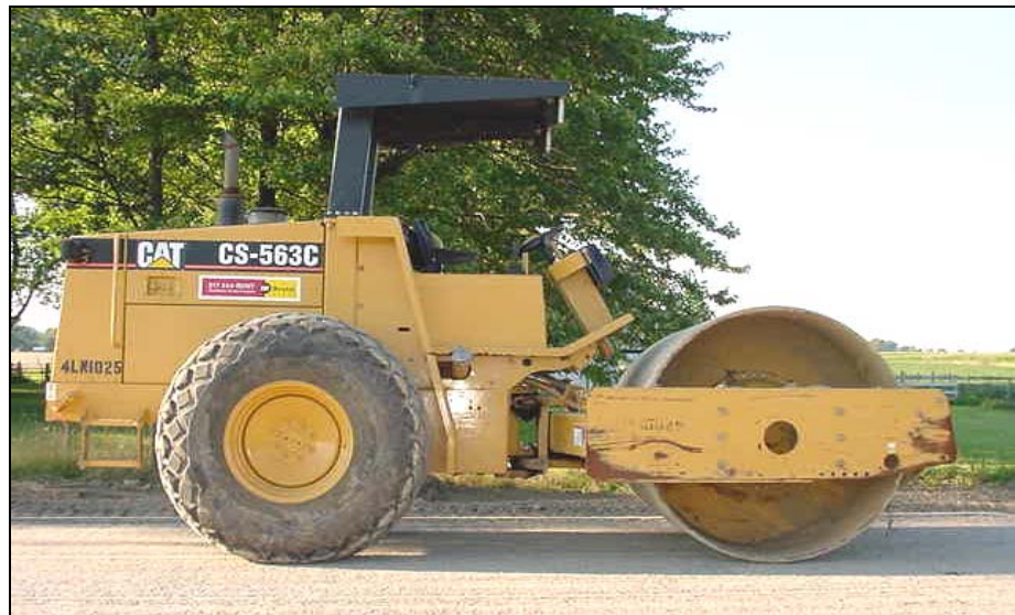
Figure 4-5. Single Drum Vibratory Roller
