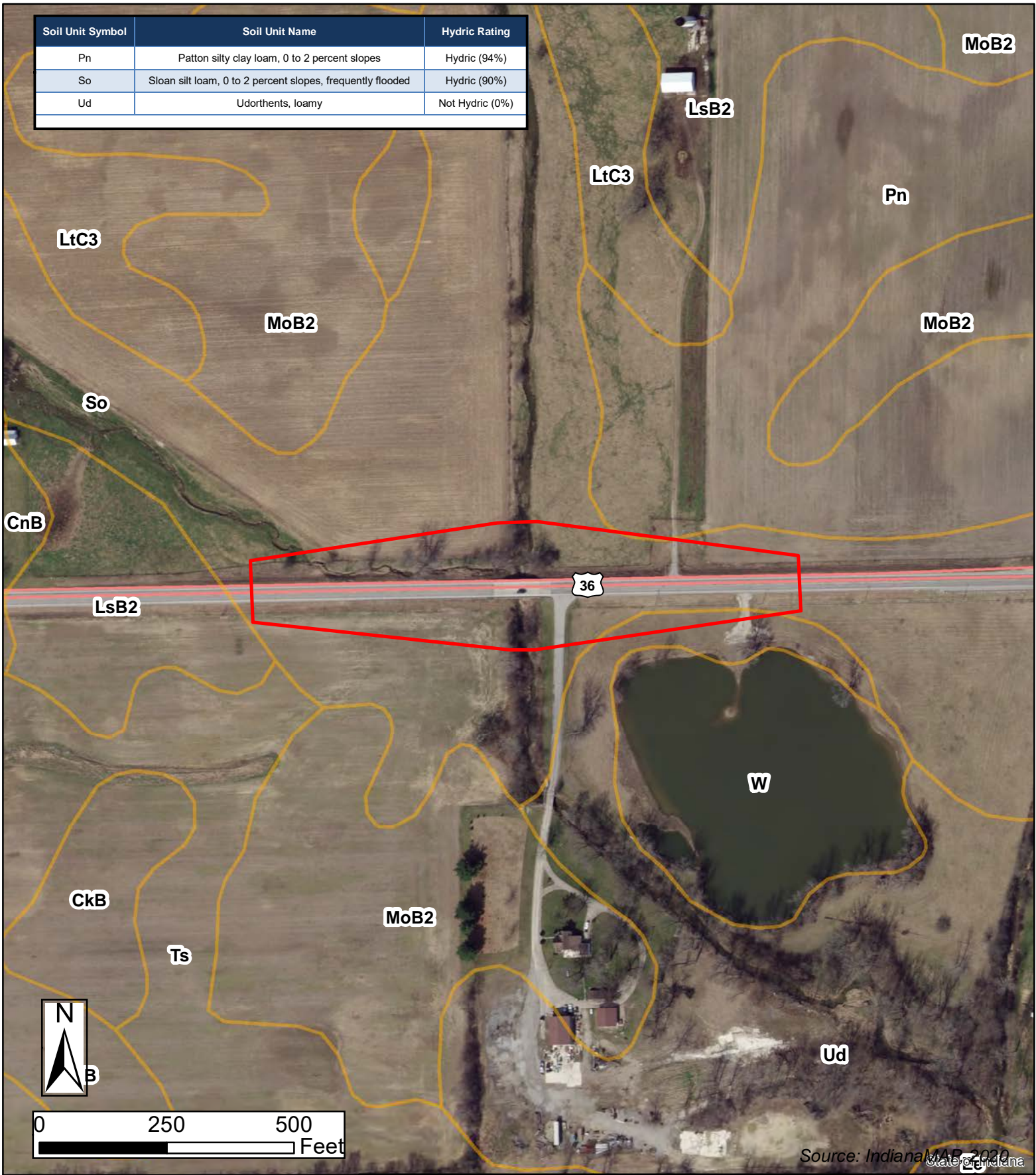
Figure 4 NRCS Soils Map US 36 Bridge Replacement Randolph County, IN Des. 1702882
