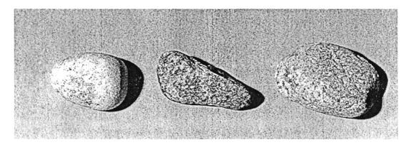
Non Fractured particle (rounded particles, smooth surfaces).
