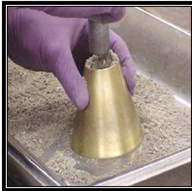
Figure 3 Tamping sand using the cone method to determine SSD
