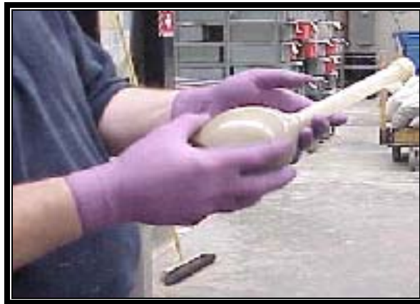
Figure 6 Agitating the pycnometer
