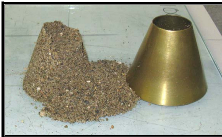
Figure 4 Sand at SSD condition will slump once the cone is removed
