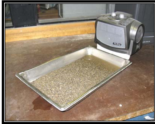
Figure 2 A current of air being used to achieve SSD condition.
