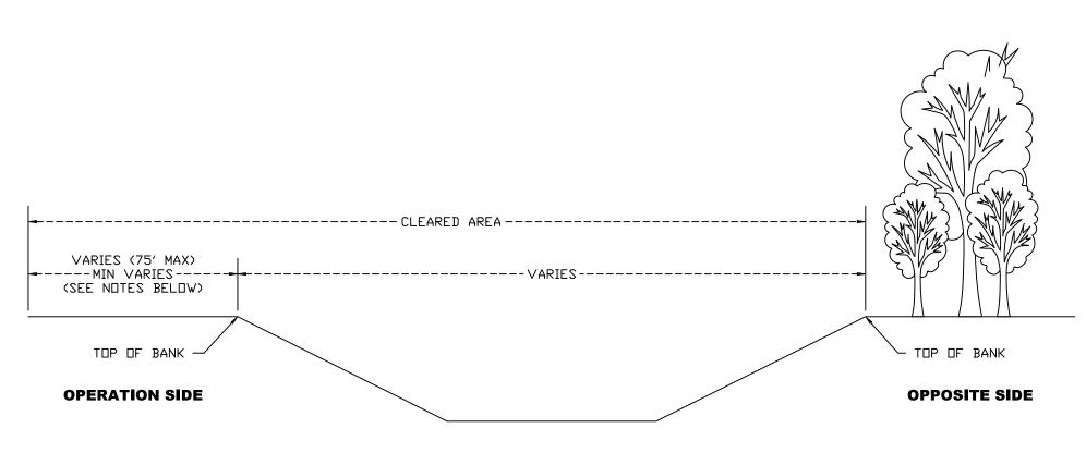
NOTE: CLEARING UNDER THIS PLAN SHALL BE DONE FROM THE TOP OF BANK TO TOP OF BANK, AS WELL AS TO A DISTANCE NEEDED TO COMPLETE CONSTRUCTION OPERATIONS ON THE OPERATIONS ON THE OPERATIONS SIDE OF THE DITCH.
