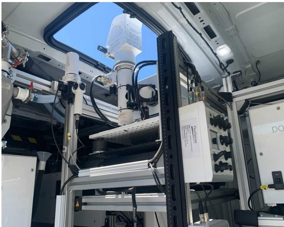
Figure A 3. The mobile SkyDOAS system: Zenith looking telescope, optical fiber and spectrometer. The SOF system is seen in the center of the sun roof.
