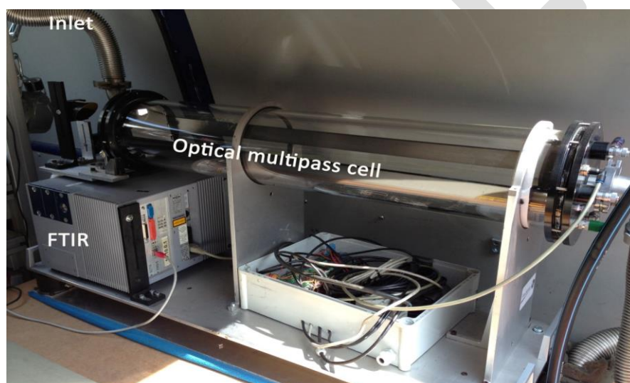
Figure A 4. The MeFTIR instrumentation consisting of a Bruker FTIR spectrometer connected to an optical multi-pass cell.
