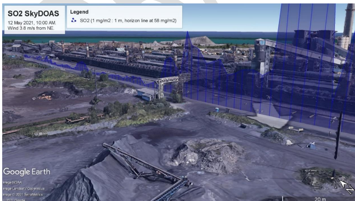
Figure 11. Example SkyDOAS measurement of SO 2 on 12 May, 10:00 AM. Winds were 4 m/s from northeast. The picture view focuses on emissions from B and D batteries, reaching a maximum column of 58 mg/m 2 , whereas the main stack plume (going through the roof of the view) reaches 748 mg/m 2 . Map from Google Earth™, 2021.
