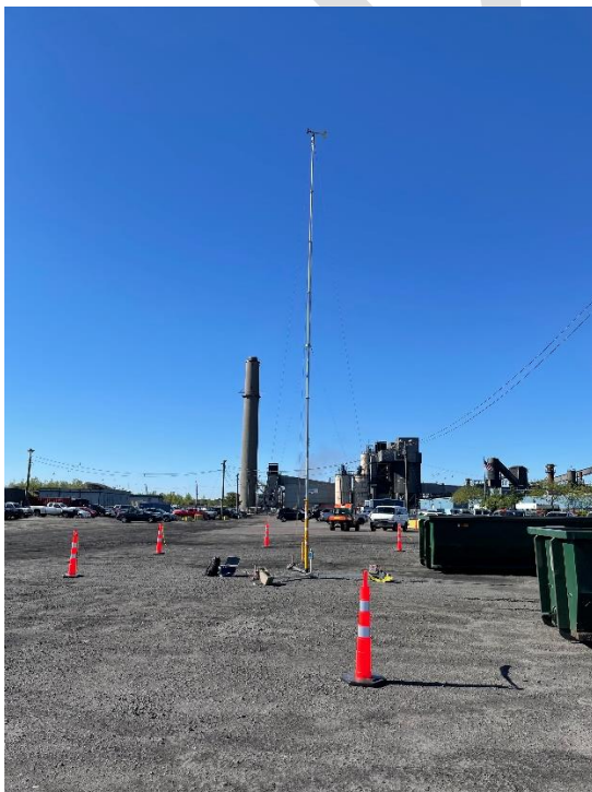
Figure A 7. The FluxSense mobile wind mast with an RM Young anemometer mounted on top. The mast was raised to 10 m height.
