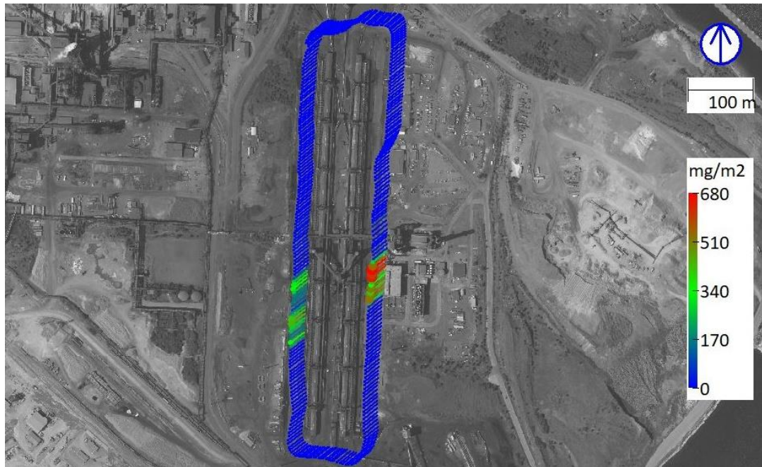
Figure 10. Example SkyDOAS SO 2 measurement 12 May 2021, 09:36-09:48 AM. Wind was blowing from northeast at 4.4 m/s as indicated by the coloured lines (pointing up in wind). The sulfur dioxide column is colour coded from background (blue) to 680 mg/m 2 . Map from Google Earth™, 2021.
