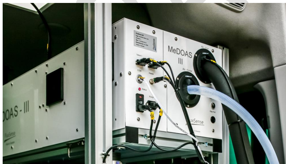
Figure A 5. The MeDOAS instrument having an overall optical path-length of up to 118 m.
