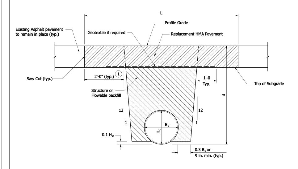
L = Pay limits of pavement removal and pavement replacement (ft); for cross pipe, measured along roadway centerline; for pipe parallel to roadway centerline, measured prependicular to pipe centerline.
