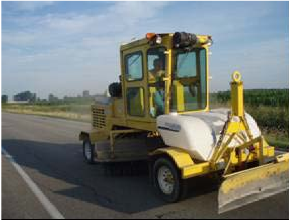
Figure 13.24-12 Rotary Power Broom
