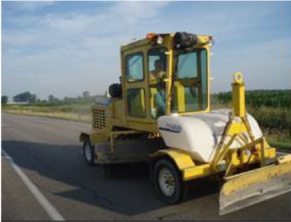
Figure 13.24-12 Rotary Power Broom
