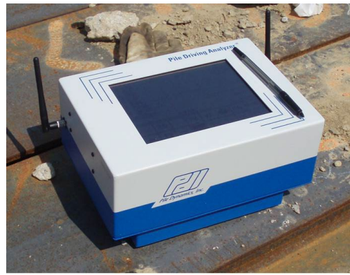
Figure 6. PDA Data Collector
