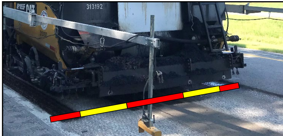
Figure 13.24-3d Spray Paver Emulsion Application Locations Red indicates front nozzle application, and Yellow indicates rear nozzle application
