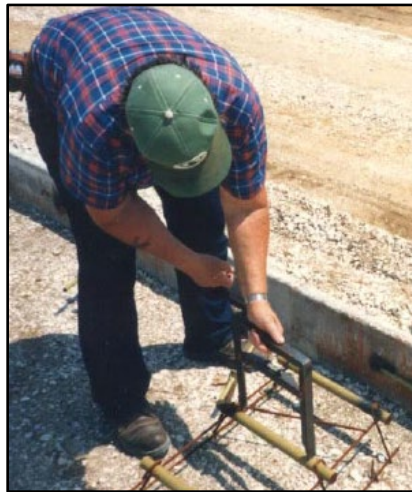
Figure 8.10.1 Dowel Bar Checker Device
