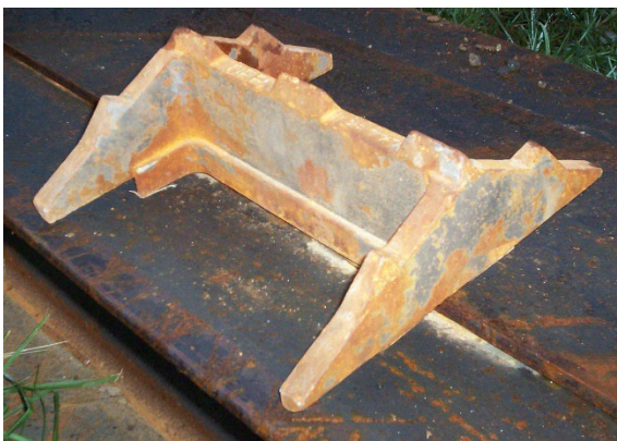
Figure 9 Bottom of H-Pile Shoe Tip
