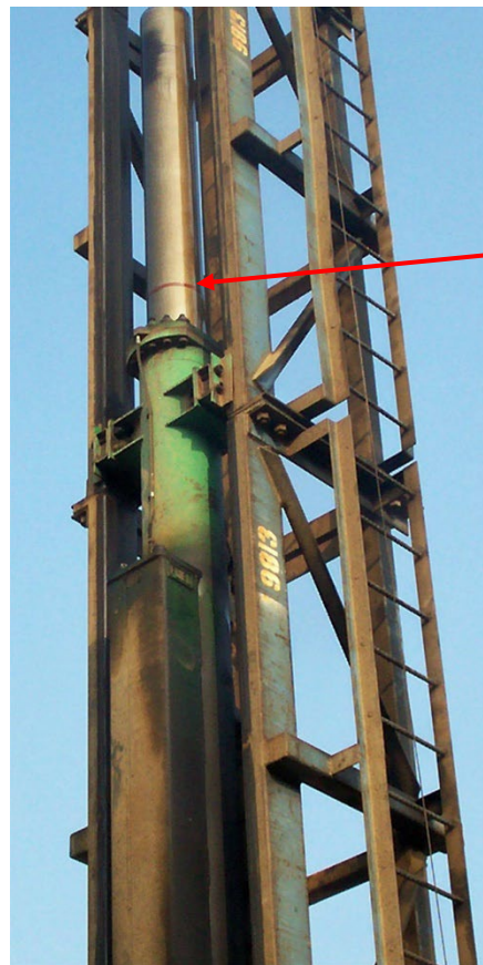
Figure 12. Piston Extending from the Top of the Hammer.
