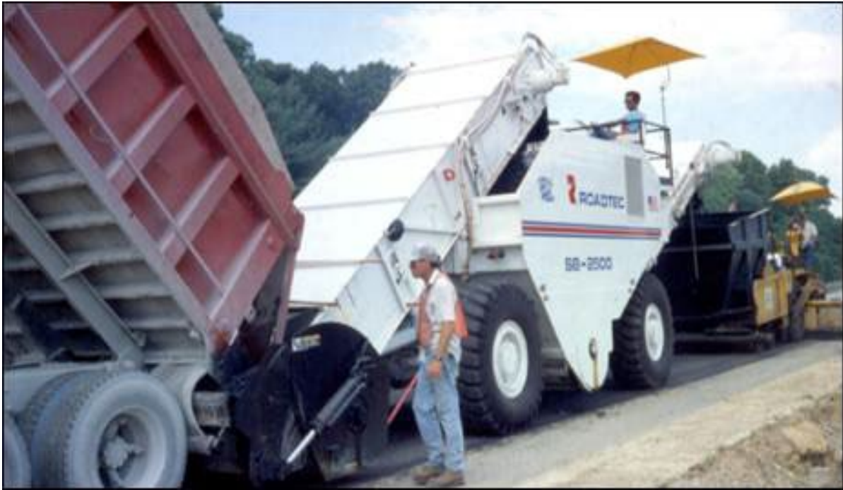
Figure 13.24-2 Material Transfer Device
