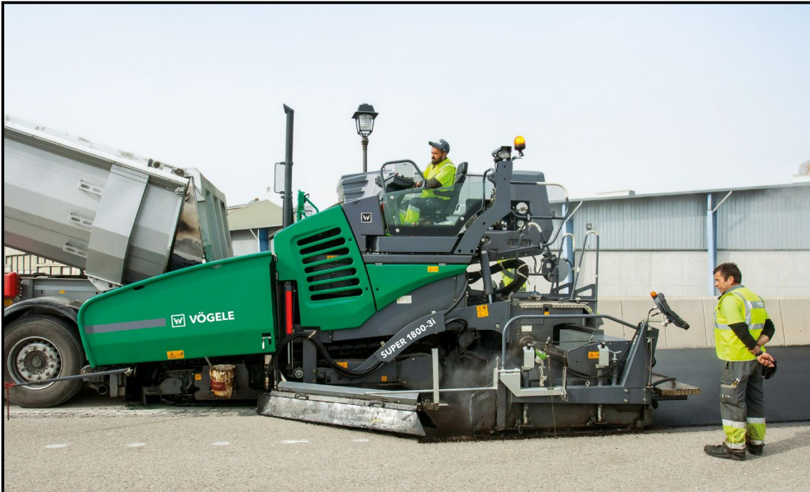
Figure 13.24-3b Typical Spray Paver
