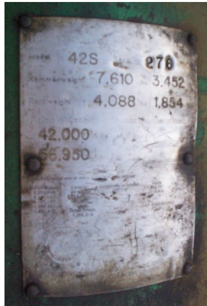
Figure 4. Pile Hammer Data Plate
