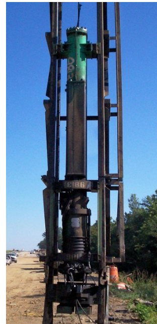
Figure 3. Photo of a Single Acting Diesel Hammer
