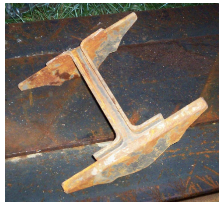
Figure 10 Top (Connection Side) of H-Pile Shoe Tip
