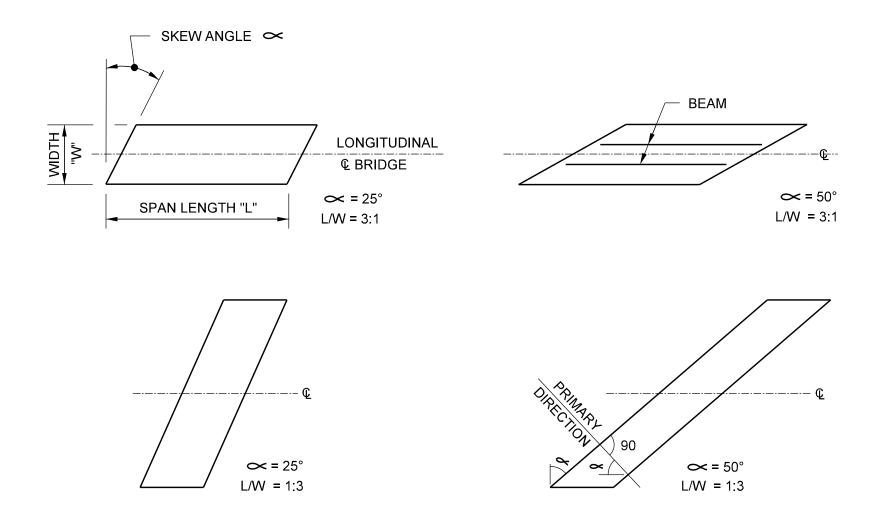
COMBINATION OF SKEW ANGLE AND SPAN LENGTH/BRIDGE WIDTH RATIO
