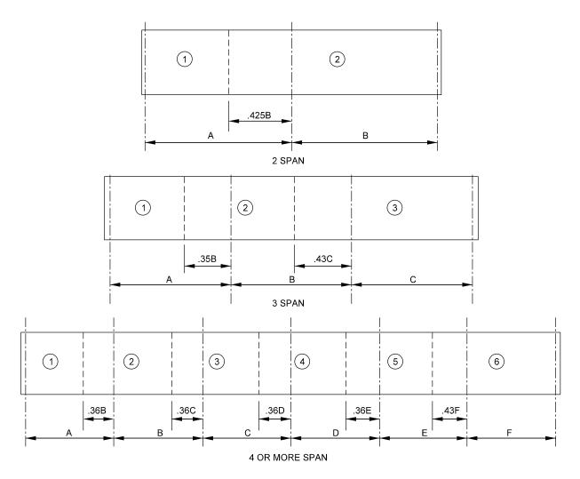
Note: Pour numbers indicate sequence of pours. Avoid placing construction joints at same location as the beam or girder splice.
