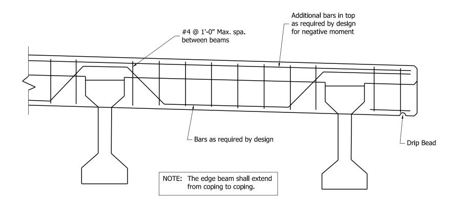
SUGGESTED ALTERNATE TRANSVERSE EDGE BEAM DETAILS (For Bulb-Tee Beam, AASHTO I-Beam, or Steel Plate Girder)
