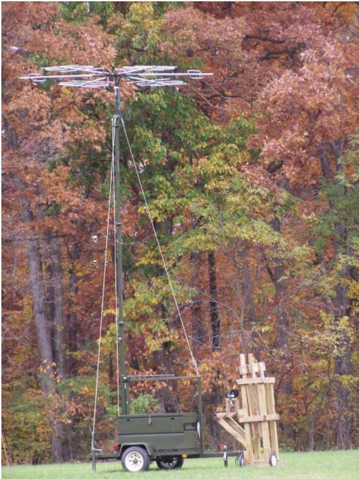
*Deployed trailer with tower and automated telemetry receiving unit.*
