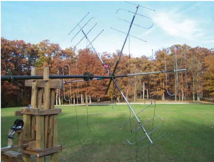
*Tower for telemetry receiving unit being assembled for deployment.*
