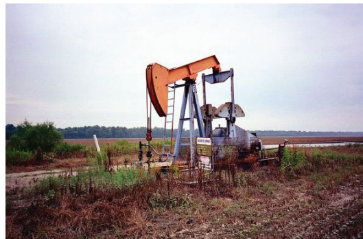
Crude Oil Pumping Unit
