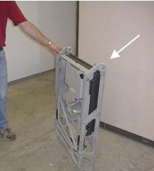
4. Carefully pull the legs away from the center. Do not force the legs open. The legs will resist further opening when they are fully opened.
