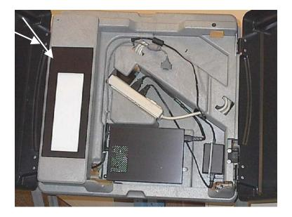
8. Place the bottom of the voting machine in the cradle at the bottom of the booth box, and carefully move the voting machine back so that it rests in the frame.
