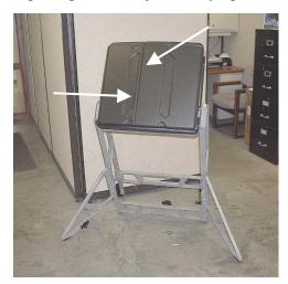
After you open the privacy screen doors, you can install the iVotronic voting machine. If you use an RTAL printer, it is already installed on the left side of the booth. If not, a blank insert is already installed on the left side of the booth.
