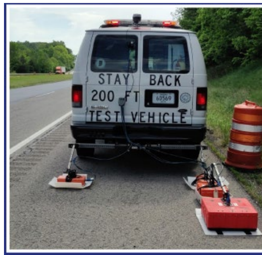
Figure 1. INDOT GPR Testing Equipment
