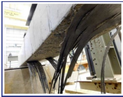
Figure 1. FRP wrap test at bridge end.
