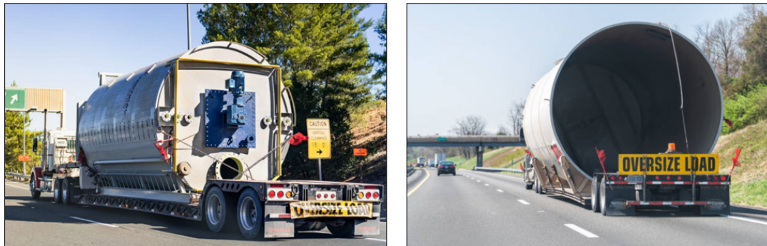
Figure 4.9 – Example Overweight Trucks (Left) and Oversize Trucks (Right)
