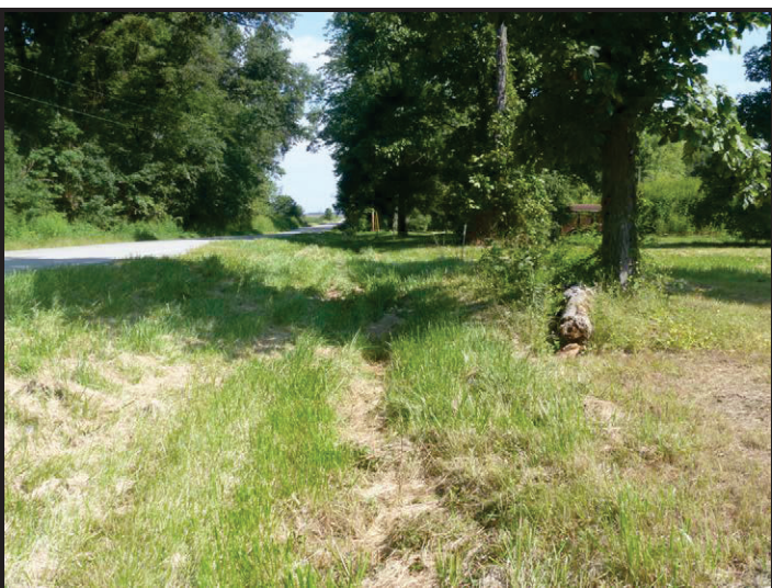
Photo 23 – Southeast Quadrant, RSD-1: Facing downgrade to the north along RSD-1 from the southern limits of the AOI. RSD-1 did not exhibit an OHWM or defined bed and bank.
