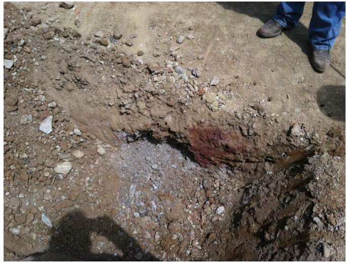
(b) Poorly mixed lime-soil modified soil
