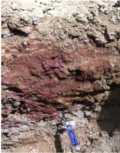
(a) Well mixed lime-soil modified soil
