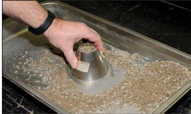
Figure 16: Excess aggregate brushed from the base
