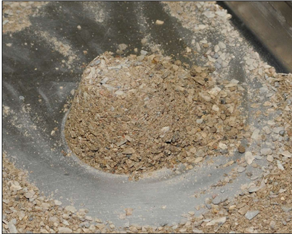
Figure 18: Sample displaying partial slump
