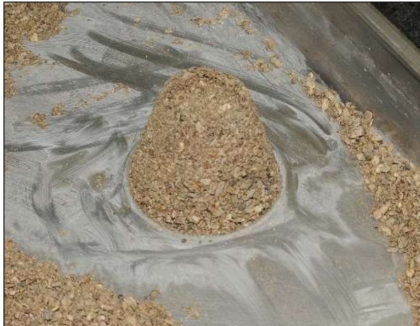
Figure 17: Sample retaining its molded shape
