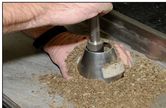
Figure 15: Tamping in a circular motion
