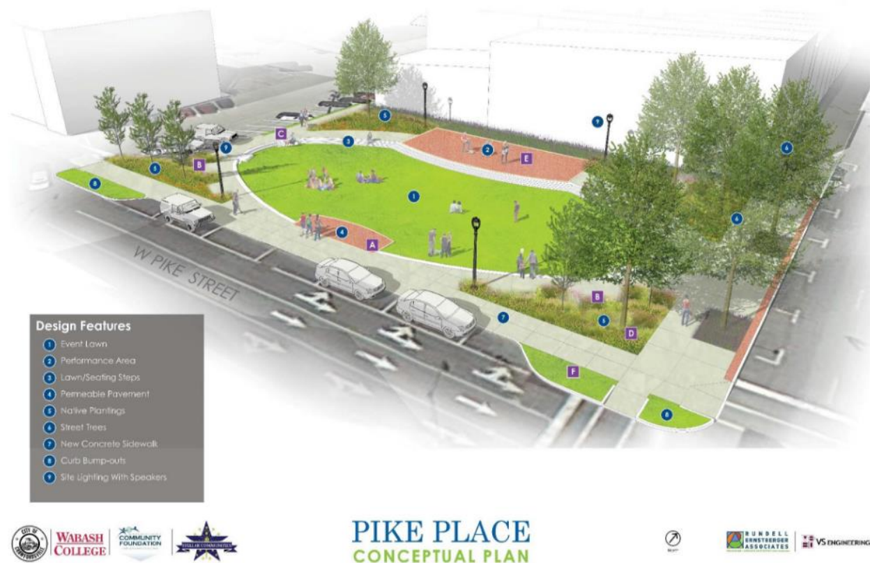
Figure 14 shows a rendering of the Pike Place conceptual plan with an event lawn, performance area, lawn seating steps, permeable pavement, native planting, street trees, new concrete sidewalks, curb bump-outs, and site lighting with speakers.
