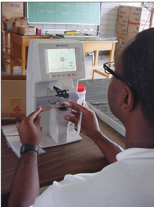
An offender uses equipment to measure and mark the strength of eye glasses.
