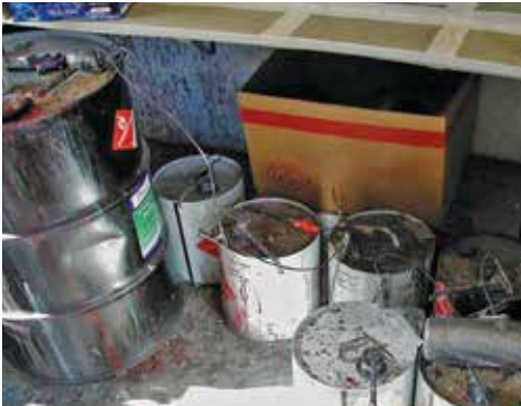
Improperly stored used oil.
