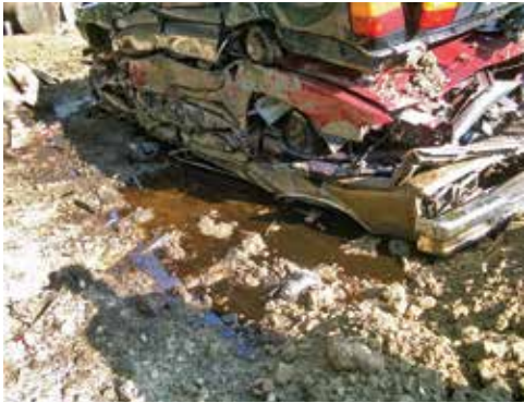
Environmental contamination from leaking crushed vehicles.
