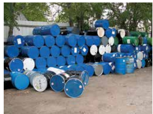
Drums capped and stored on their sides.
