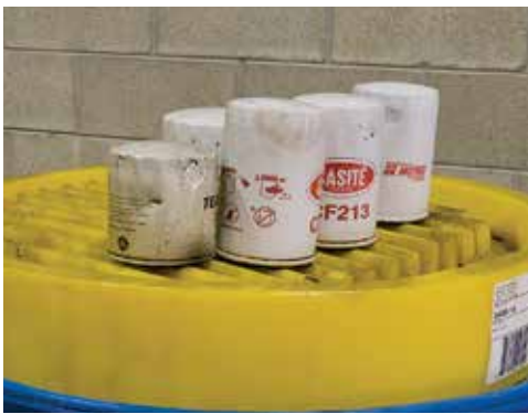
Oil removed and drained from oil filters.
