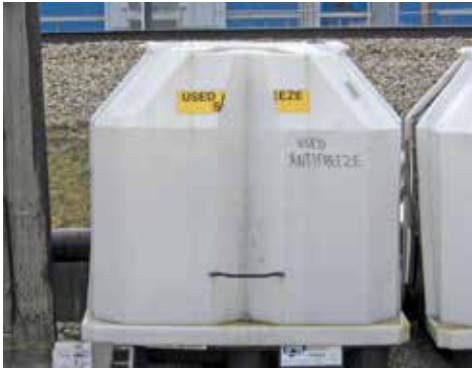
Properly labeled and stored antifreeze.
