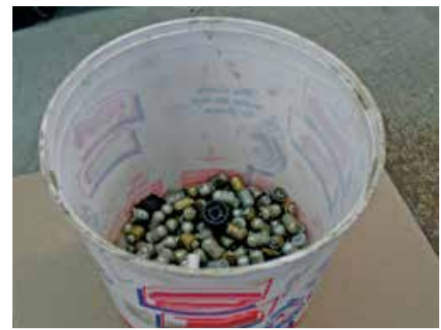
Improper mercury switch storage.
