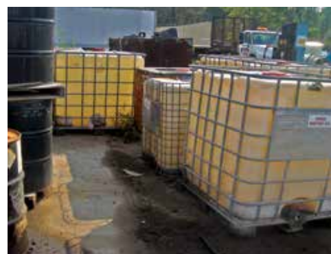
Oil storage capacity exceeding 1320 gallons.
