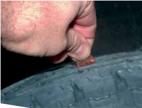
2/32 inch tread depth test with a penny.
