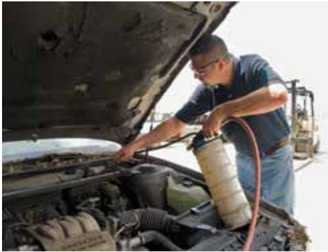
Removal of fluids prior to storing the vehicle.
