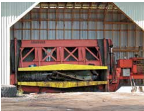
Crusher placed in secondary containment.
