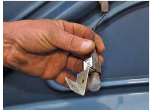
Removal of a light containing a mercury switch.
