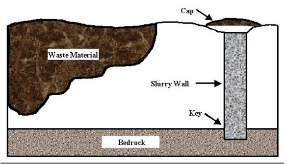
**Picture from** https://frtr.gov/matrix2/section4/D01-4-53.html The slurry wall key must be either into bedrock or a layer of appropriately low permeability.
