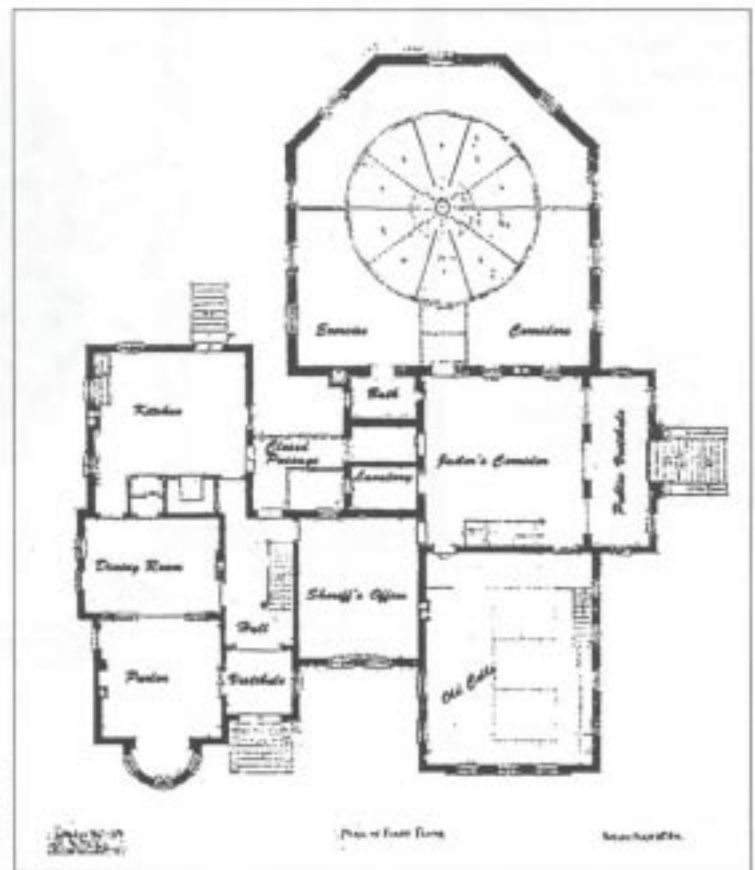
The Pauly Co. catalog includes typical floor plans for a rotary jail and sheriff's residence. This reproduction shows the first floor plan of a structure.
